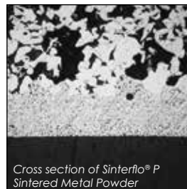
Magnification of Sinterflo® P Sintered Metal Powder
