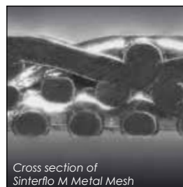
Magnification of Sinterflo M Metal Mesh
