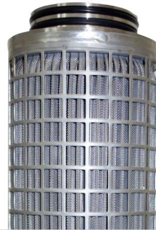
The Compfil™ PF filter consists of a regenerable, pleated filter tube made of stainless steel. Due to its robust construction, the Compfil™ SF is designed for maximum differential pressures up to 10 bar. It can be used in a temperature range from -20-210°C without any problems. From a temperature of 180°C, however, special O-rings are required.
