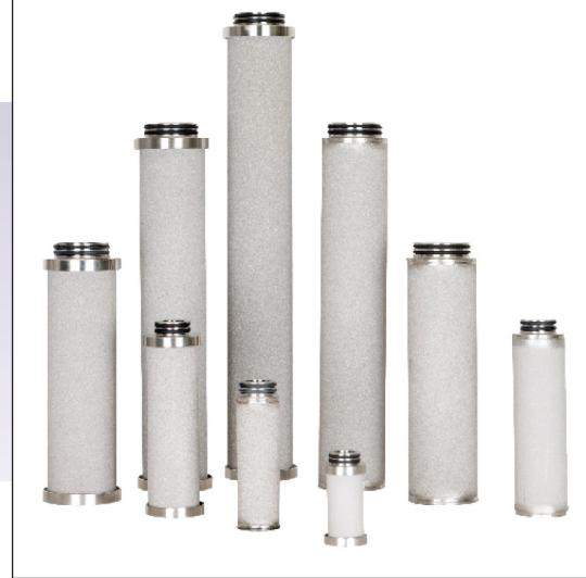
The Compfil™ SF filter is designed for removal of particles from gases, liquids and steam. The SF consists of a re-generable isostatically pressed filter cylinder made from sintered stainless steel. The retention rate ranges from 1µm to 25µm.
