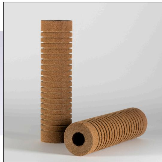
**Bonfil™** is a resin bonded filter that is constructed using an advanced manufacturing process producing a rigid graded density filter. The rigid phenolic resin structure ensures that our Bonfil™ filters can withstand high viscosities and temperatures without deformation or collapse of the pores.
