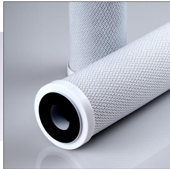
The Carbofil™ series is the new generation of carbon cartridges produced by the extrusion process. They provide long service life and superior adsorption performance compared to conventional granular activated carbon cartridges together with minimum fines. With a high mechanical strength and low ash content, the carbon block structure prevents channelling, bypassing, fluidizing or unloading of carbon fines.
