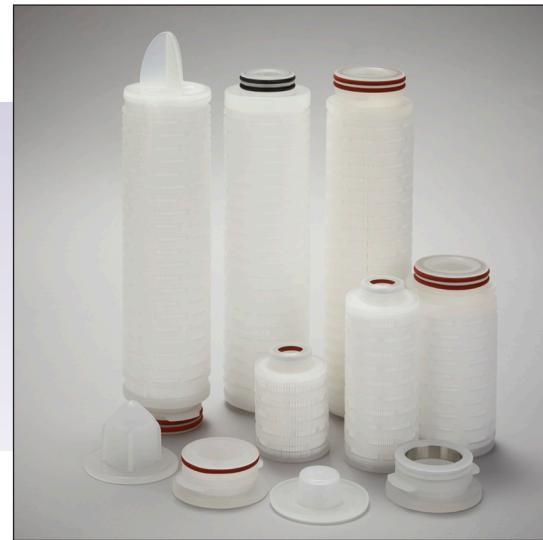
Fluorofil™ F100 cartridges are manufactured using a highly hydrophobic 1 micron PTFE membrane. The enhanced PTFE membrane offers exceptionally high liquid flow rates at low pressure differentials, making Fluorofil™ F100 cartridges ideally suited to solvent filtration.
