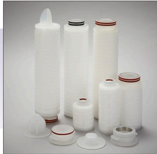
A range of absolute rated cartridge filters are manufactured, featuring the latest developments in borosilicate glass fibre filter media technology; Microfil™ cartridges are constructed from robust glass fibre and polypropylene filtration layers, offering removal ratings from 0.5 to 5 micron absolute.
