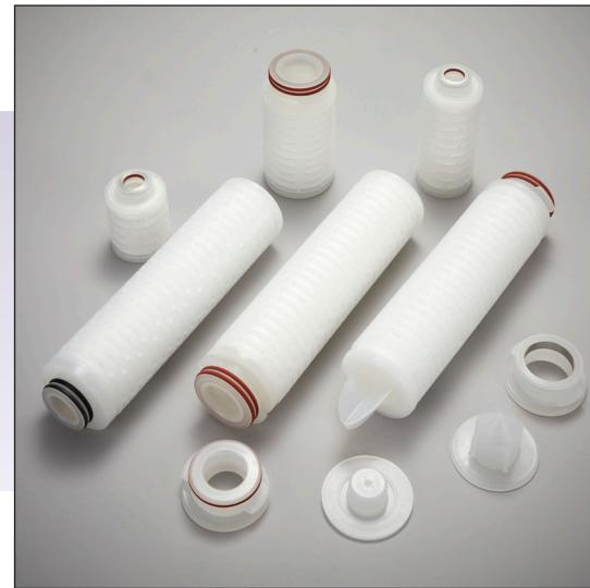
**Biofil™ 2 cartridges are based on a naturally hydrophilic polyethersulfone (PES) membrane with a mirrored asymmetric pore structure. When combined with quality all-polypropylene cartridge components and high integrity manufacturing techniques, the polyethersulfone membrane provides a high strength, long life cartridge of consistently precise microbial retention.**
