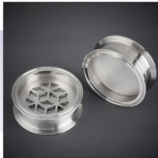
**Sinterflo® CRC** multi layered, diffusion-bonded stainless-steel meshes are available in 316/316L and other alloys. This precision filter mesh, also known as a porous plate, is available in a range of different pore sizes ranging from 1 - 100 microns in various diameters.
