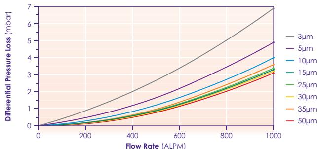
\* Using a 10" element. Water and air at ambient temperature and 1 bar (A). Steam is dry saturated steam at 1bar (A).
