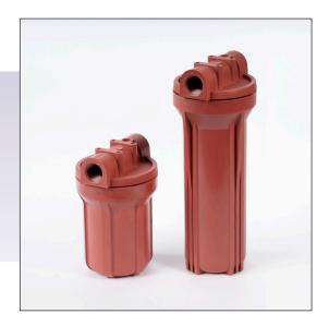
The following units consist of a 5 micron fine particle removal cartridge in a glass reinforced nylon housing for hot water/high pressure applications. These filters can withstand temperatures to 180°F and pressures to 200 psi. They have the same sediment removal capabilities as our standard sediment units.
