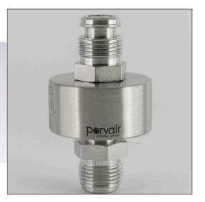
GasPro<sup>™</sup> TEM-3780 Series sintered nickel media filters are designed for filtration of UHP semiconductor gases where a compact, all-metal, corrosion tolerant design is required. This all-welded assembly will deliver 3 nm particle retention, where a high flow rate and low pressure drop is required and where space is limited. Standard semiconductor industry fittings are offered for easy installation.
