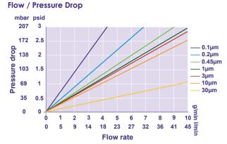
Flow rates shown are for a nominal 10" (254mm) long cartridge. For fluids other than water, multiply the pressure drop by the fluid viscosity in centipoise.
