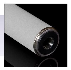
Sinterflo® P is a robust material manufactured from sinterbonded metal powders. Primarily produced in 316/316L grade for use in temperatures up to 420°C (788°F), depending on process conditions, and offering resistance to most chemicals, Sinterflo® P media can also be produced in other grades of stainless steel and alloys such as Inconel®, Hastelloy® and Monel®.
