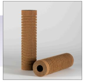
Bonfil<sup>™</sup> is a resin bonded filter that is constructed using an advanced manufacturing process producing a rigid graded density filter. The rigid phenolic resin structure ensures that our Bonfil<sup>™</sup> filters can withstand high viscosities and temperatures without deformation or collapse of the pores.
