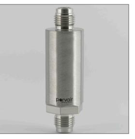
GasPro™ TEM-900 series filters are designed for 3 nm particle retention up to flow rates of 30 slpm and temperatures up to 121°C (250°F)
