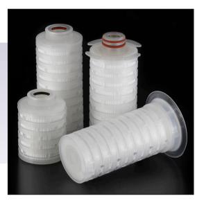
Biofil™ Junior cartridges are based on a naturally hydrophilic polyethersulfone membrane with a mirrored asymmetric pore structure. When combined with quality all-polypropylene cartridge components and high integrity manufacturing techniques, the polyethersulfone membrane provides a high strength, long life cartridge of consistently precise microbial retention.
