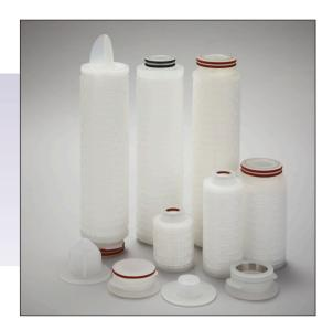
Fluorofil<sup>TM</sup> F100 cartridges are manufactured using a highly hydrophobic 1 micron PTFE membrane. The enhanced PTFE membrane offers exceptionally high liquid flow rates at low pressure differentials, making Fluorofil<sup>TM</sup> F100 cartridges ideally suited to solvent filtration.
