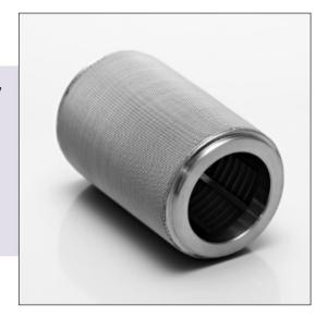
This is a digital inkjet filter specifically designed for use on super-wide format printer platforms. The filter is engineered from high grade stainless steel and has various micron rating options. A resistance weld manufacure process gives the filter added durability, and the stainless steel mesh filter media ensures an extended lifespan and excellent through flow.
