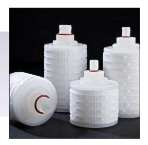
Ventafil™ cartridges are manufactured using a highly hydrophobic ePTFE membrane and are designed for autoclave venting. The enhanced ePTFE membrane offers exceptionally high gas flow rates at low pressure differentials.
