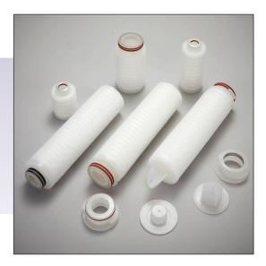
Vinofil™ membrane cartridges are specifically designed for wine and beer filtration, as a final filter for cold biological stabilisation. Vinofil™ cartridges utilise a double layer of naturally hydrophilic polyethersulphone (PES) membrane with a mirrored asymmetric pore structure, providing graded filtration throughout its depth, resulting in higher throughputs and long service life.
