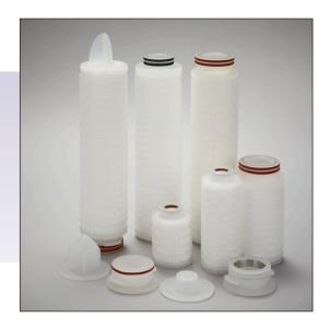
Hydrofil™ Plus microbial rated cartridges have been developed and manufactured for the filtration of liquids in the pharmaceutical, biotechnology and other critical applications. Hydrofil™ Plus utilises a naturally hydrophilic Nylon 6.6 membrane with a mirrored asymmetric pore structure. The cartridge's unique built in pre-filtration membrane layer provides longer life and higher throughput.
