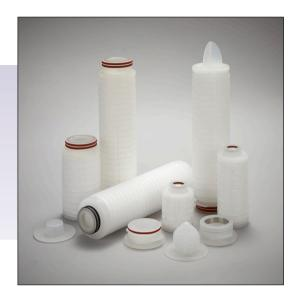
Superior filters made of high quality PES (Polyethersulfone) membrane with low pressure drop, high flow rate and long service life for direct DI water, TMAH developer, weak acids and base solutions.
