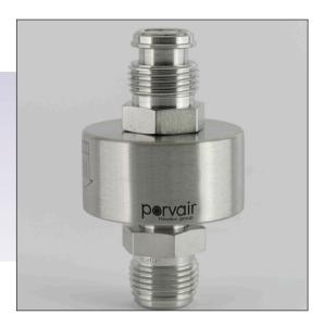
GasPro<sup>TM</sup> TEM-3790 Series sintered nickel media filters are designed for filtration of UHP semiconductor gases where a compact, all-metal, corrosion tolerant design is required. This all-welded assembly will deliver 3 nm particle retention, where a high flow rate and low pressure drop is required and where space is limited. Standard semiconductor industry fittings are offered for easy installation.
