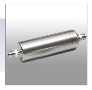
GasPro<sup>TM</sup> TEM-1400 Series filters are designed for 3 nm particle retention up to flow rates of 75 scfm and temperatures of 150°C (302°F).
