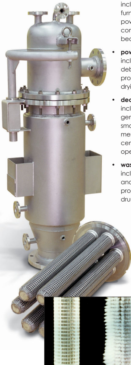
Figure 1 Moving across the photograph from left to right: the metal fibre element loaded with dust; the dust is removed from the surface by the pulsed jet action; the dust is carried away; the dust begins to settle; and quickly falls to the bottom of the vessel leaving a clean element. The sequence time is less than half a second. The cleaning pulse is made whilst process flow continues.
