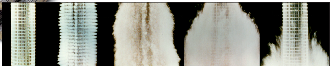
Figure 1 Moving across the photograph from left to right: the metal fibre element loaded with dust; the dust is removed from the surface by the pulsed jet action; the dust is carried away; the dust begins to settle; and quickly falls to the bottom of the vessel leaving a clean element. The sequence time is less than half a second. The cleaning pulse is made whilst process flow continues.
