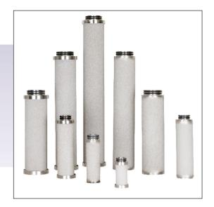
The Compfil<sup>TM</sup> SF filter is designed for removal of particles from gases, liquids and steam. The SF consists of a re-generable isostatically pressed filter cylinder made from sintered stainless steel. The retention rate ranges from 1µm to 25µm.
