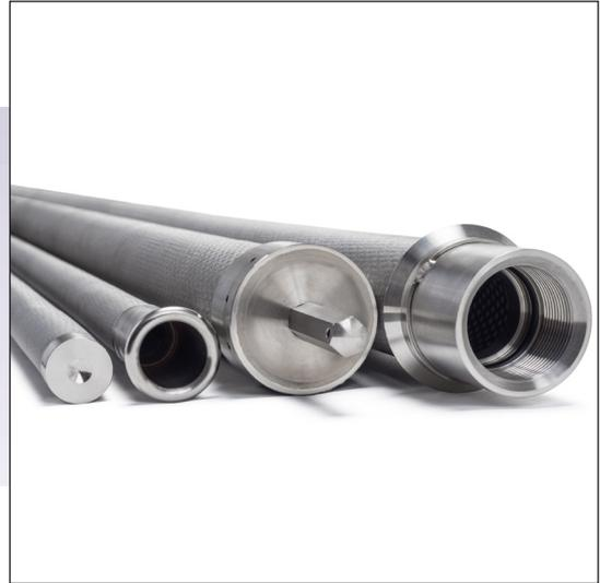
Our septa filter elements are made from Sinterflo® mesh composite (MC) filter media. This unique material is made from wire mesh and perforated metal, sintered together into a durable porous filtration medium.
