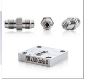
GasPro RFPs (restrictive flow products ) are sintered porous metal flow restrictors with hundreds of micropores. These are clog resistant, flow limiting devices used to deliver highly acurate flow of high-purity speciality gases or limit the flow of compressed semiconductor process gases.
